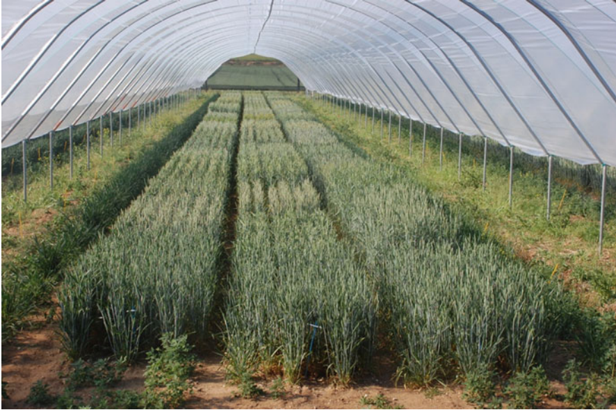
Fig. 3.3 Large polytunnel rainout shelters used to apply managed drought conditions in the field. Shown are plots of 66 wheat genotypes grown at Broom's Barn, Suffolk, UK. The cost-effective facility allows control over the timing and severity of the water deficit with minimal impact on crop microclimate (Ober et al. 2010)
